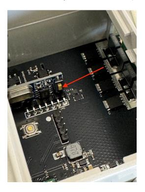
The indicator LED on the receiver (see arrow) will light up. The receiver is now in learning mode. Press and hold any button on the remote control for at least 3 seconds. The indicator LED on the receiver will turn off.
